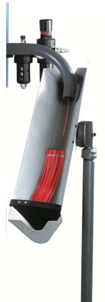
The 48" Wire Collector is a pedestal-mounted, V-shaped trough for collecting short wires produced by an automatic stripper. A rubber wire stop in the trough can be adjusted quickly to handle different wire size lengths. The sides of the troughs slope at a 45° angle for easy wire removal. The height is adjustable as also the trough pivot degree.
