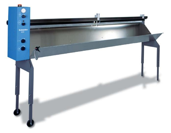
The Model 6650 Wire Stacker is designed to work with Eubanks air-powered automatic wire strippers. It will stack wires from 12 in to 96 in long and operates equally well with both small and large, wire. Feed rolls pick up the wire as it leaves the wire stripper and feeds it into a closed channel.
