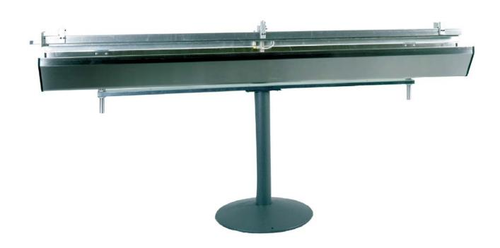
The Model 6610 Automatic Wire Stacker is designed to complement all Eubanks AutoStrip wire strippers. It is simple and highly efficient. The AutoStrip's wire ejection belts feed the wire into the stacker's gate. When the wire is cut, a pneumatic pulse from the AutoStrip opens the gate permitting the wire to fall into the collection trough. No electric power is required. A pneumatic tube is the only connection to the wire stripper.
