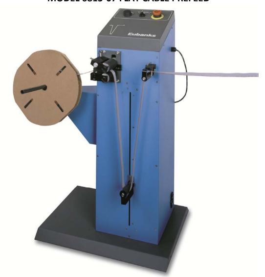
The 6815-07 Flat Cable Prefeed is designed exclusively for the Eubanks Model 4600 Cutter. It will handle Ribbon cable, Shrink Tubing, Nylon braids, Copper braids, Thin Flat Copper, or any other soft flat material that is rolled in a spool. The 6815-07 can support on its built-in arm a spool or reel weighing up to 60 Lbs (54kg).
