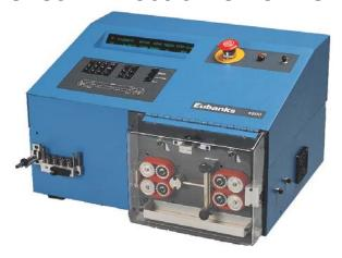
The Model 4900 is a compact AutoStrip, a small machine with big machine performance. Like its stable mates, it will cut and strip wire as small as 32 AWG (0.03mm<sup>2</sup>). It will handle wire as large as 10 AWG (6mm<sup>2</sup>), and flat cable and multi-conductor cable up to 1/4" (6mm) in diameter or width.
