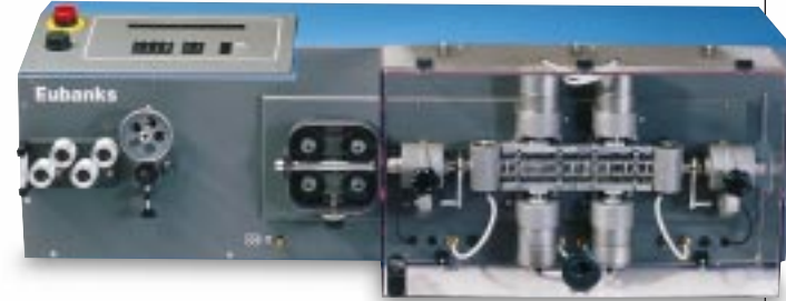
Special tandem cutterhead enables combined strip lengths of up to nine inches (229mm) in normal mode and a strip length of up to 100 in. (1,000mm) on the leading end in step-strip mode.
